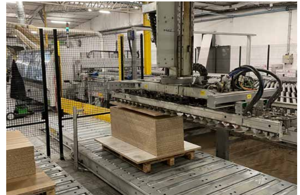
Automatic loading/unloading system used on the worktop edge banding line
